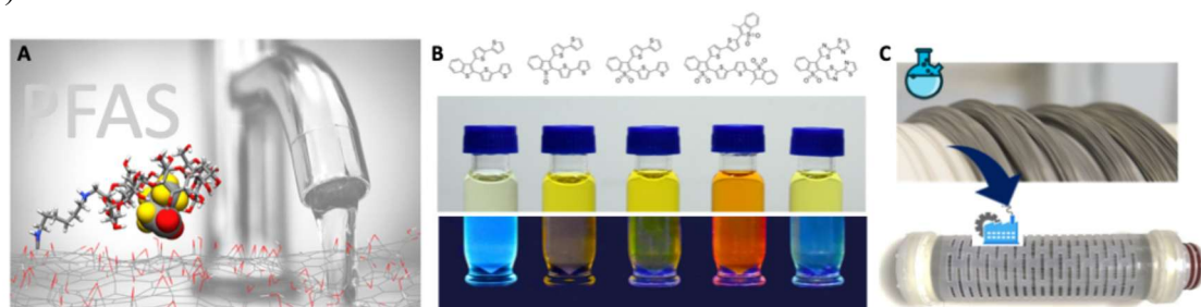
Figure 1. a) ECs monitoring and removal from drinking water: b) tailoring oligothiophene based photocatalysts 1 for ECs degradation, c) graphene oxide-polysulfone membranes and filters from lab to fab. 4,5
